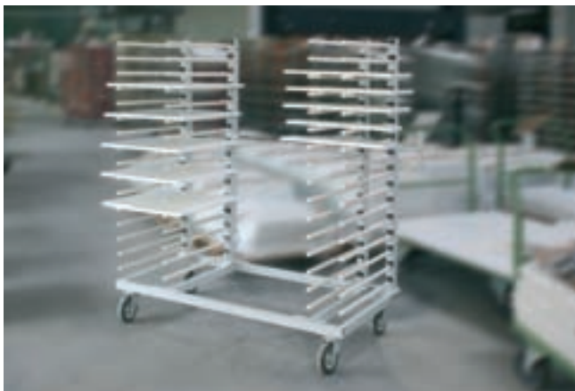
Transport trolley HWV for storage and transport of workpieces
