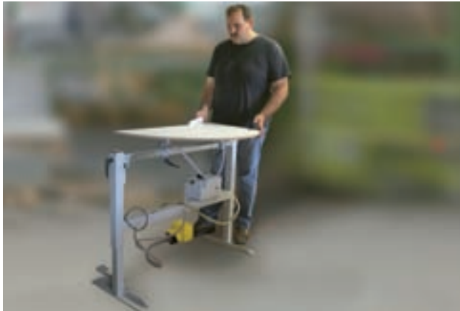
Vacuum workbench for machining of sheets of wood
