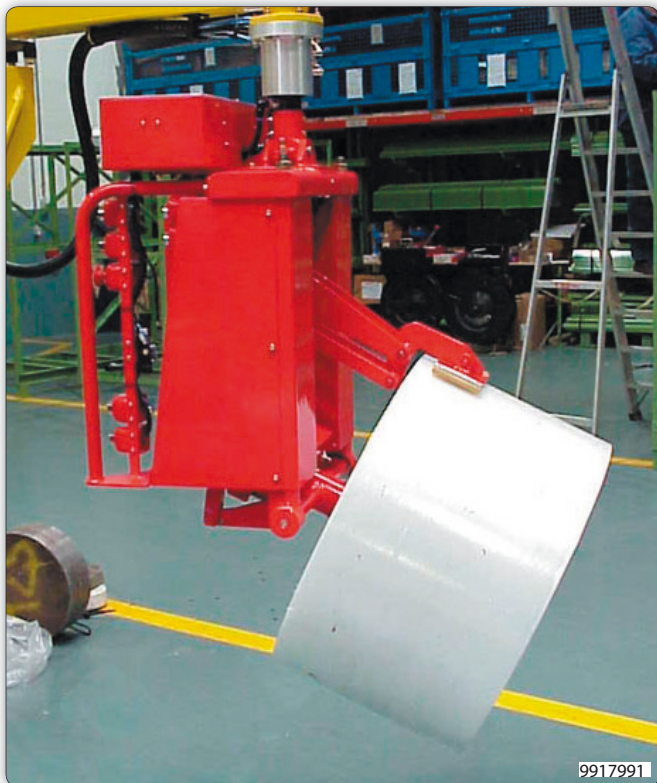
Manipulator fitted with expanding mandrel and anti-telescoping device. The tooling also incorporates 90° pneumatic inclination.
