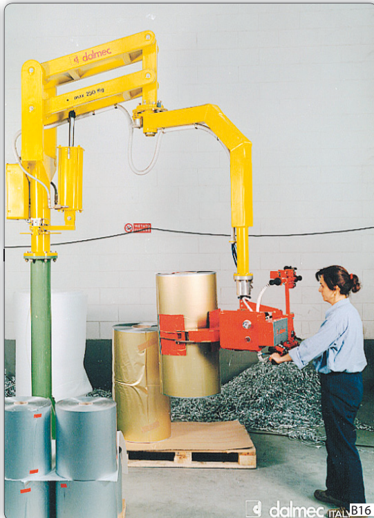
PMC type Partner manipulator, column mounted, with gripper tooling, for handling reels about their external diameter, with pneumatically assisted rotation through \pm 90^\circ .
