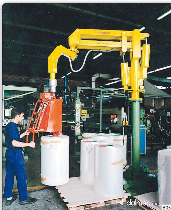
PMC column mounted manipulator custom-built for lifting reels of plastic film from a cradle to a pallet.
