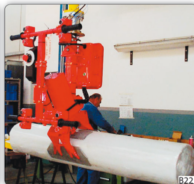
Manipulator with pneumatic gripping jaws for the easy picking of stacked reels about their external diameter.
