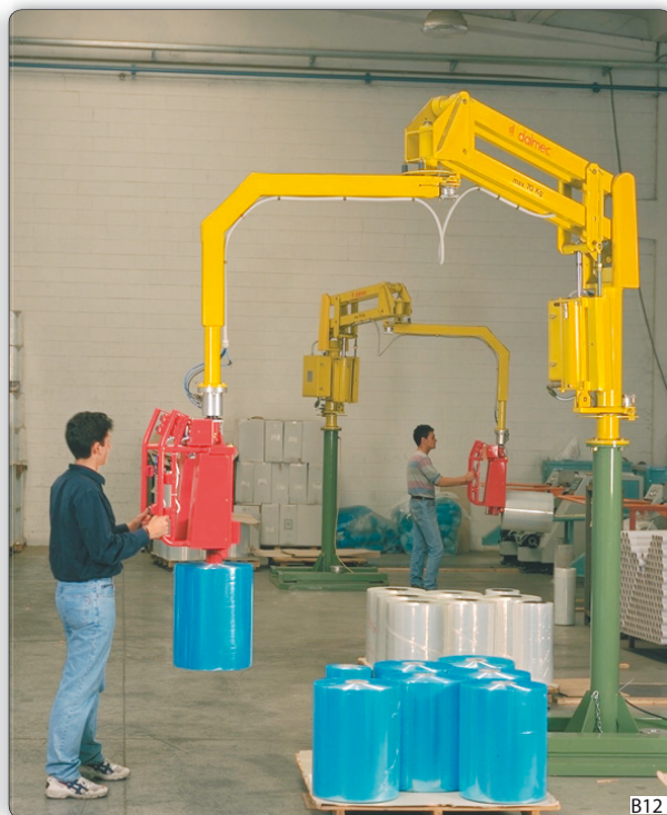
PMC type Partner manipulator, column mounted, fitted with pneumatic mandrel tooling for gripping in the reels core and 90° inclination. The unit is used for palletizing reels.
