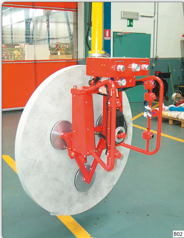
Manipulator with vacuum suction head and pneumatic 90° inclination for handling reels of cardboard. Vacuum is generated by a multi-stage "Venturi" type ejector.
