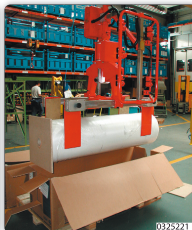
Adjustable jaws tooling for handling reels and their packaging.
