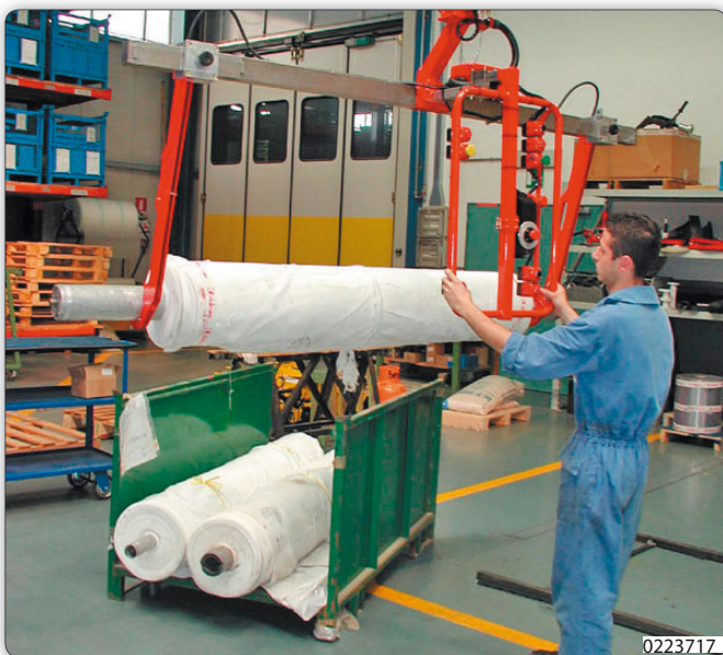
Manipulator with adjustable forks type tooling for handling of reels.
