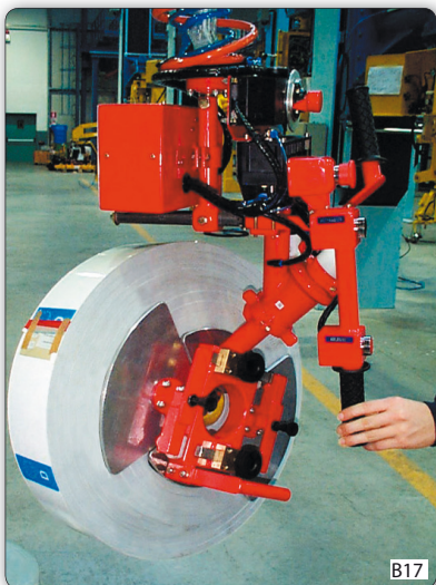
Manipulator with "Venturi" suction cups tooling for gripping reels, with manual rotation from horizontal to vertical.
