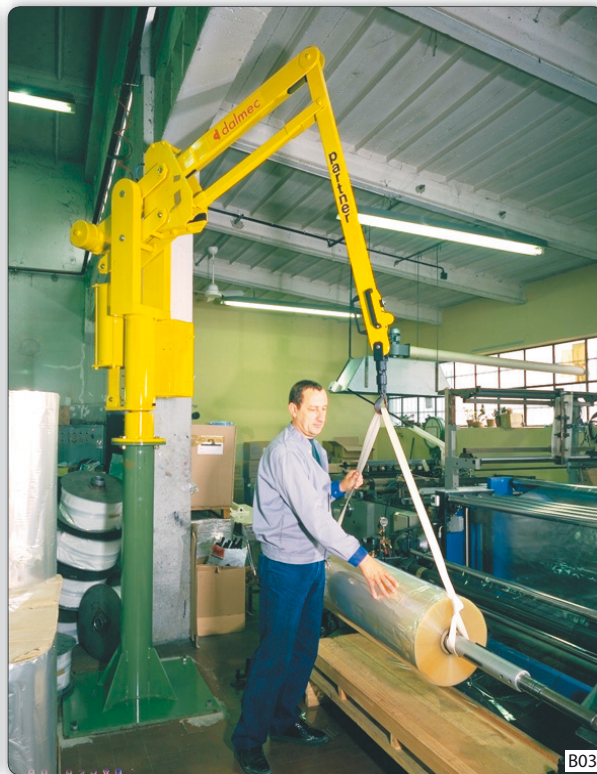
PSC column mounted Partner manipulator, standard hook unit fitted with sling by the customer for handling reels.
