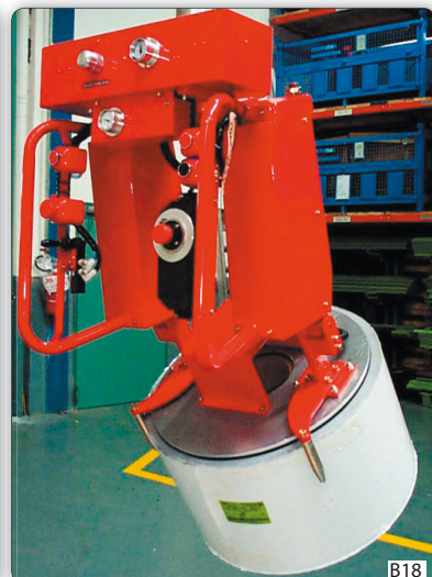
Manipulator with "Venturi" vacuum suction ring and 90^\circ pneumatic inclination.
