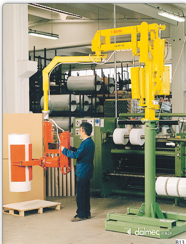
PMC type Partner manipulator, column mounted, with self-centering grippers for moving reels of plastic film. The tooling head is designed to pick horizontal reels from a winding shaft and then place them vertically to an adjacent pallet. Rotation is actuated pneumatically.
