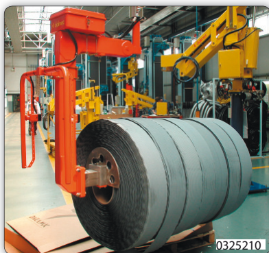
Gripping tooling with pin for handling rolls.
