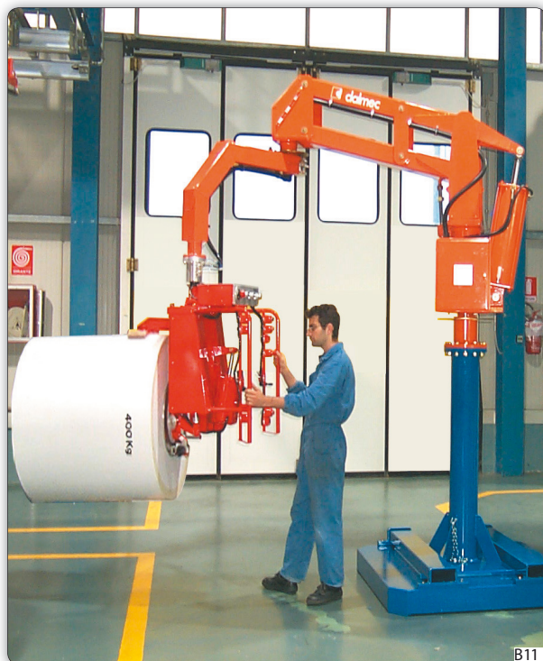
MXC type "Maxipartner" manipulator, column mounted. The tooling is equipped with an expanding mandrel, 90° pneumatic inclination and also an anti-telescoping device.
