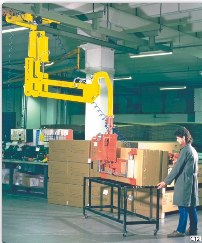
PMS type Partner manipulator, overhead trolley mounted, with motorised pneumatic drive, equipped with special gripper tooling, which allows the operator for gripping and 90° inclination of the box, so that pins can be fitted under the same. It is also completed with tracking system made by Dalmec.
