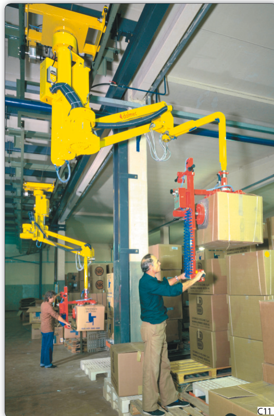
PMS type Partner manipulator, overhead trolley mounted, with motorised pneumatic drive, equipped with special suction head and telescopic commands to allow the operator to pick boxes from a high stack on a pallet.
