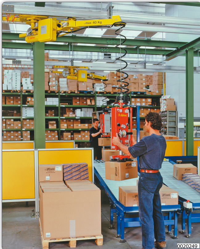
SPS type Speedyfil manipulator, overhead trolley mounted, equipped with a Venturi vacuum suction system.
