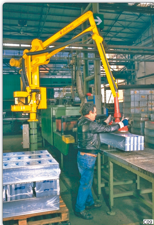
PSC type Partner manipulator, column mounted, fitted with suction cups tooling for gripping shrink-wrapped goods from a packaging line to a pallet.
