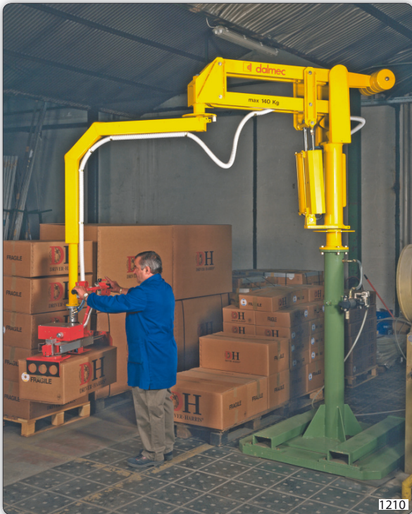
PMC type Partner manipulator, column mounted, equipped with jaws gripping system, for the palletization of packing boxes.
