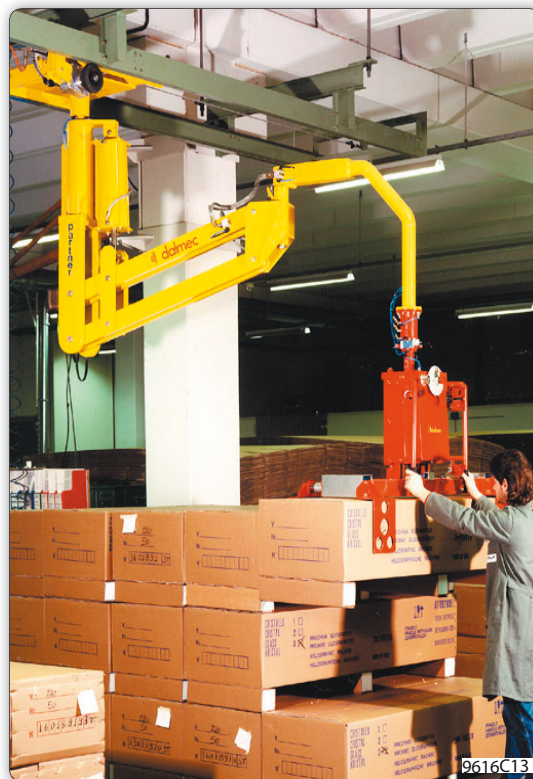
PMS type Partner manipulator, overhead trolley mounted, with motorised pneumatic drive, equipped with special gripper tooling, which allows the operator for gripping and 90° inclination of the box, so that pins can be fitted under the same. It is also completed with tracking system made by Dalmec.
