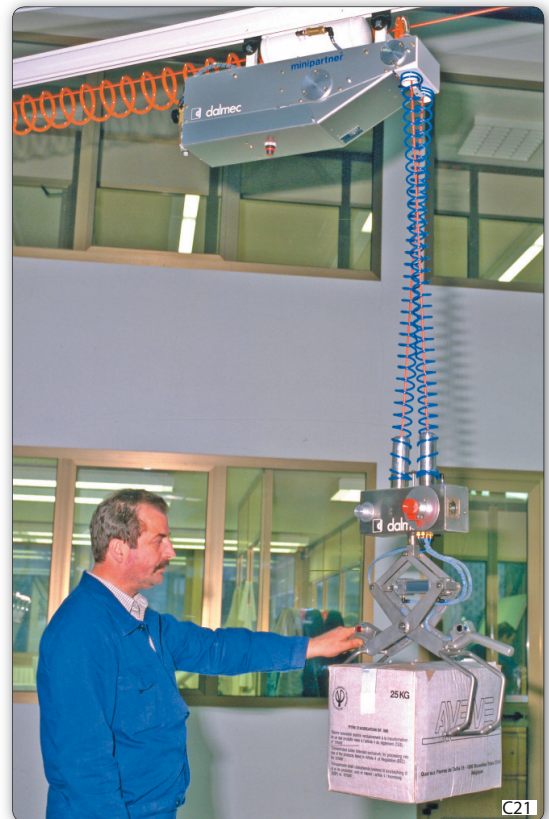
MPS type Minipartner manipulator, with overhead balancer unit, handling blocks of butter, both with and without packaging. The tooling is made of stainless steel, and the pneumatic grippers are controlled by a pressure regulator.
