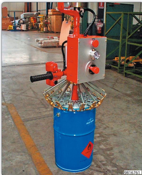
Manipulator equipped with pneumatic tooling for closing and gripping pails on the upper edge.
