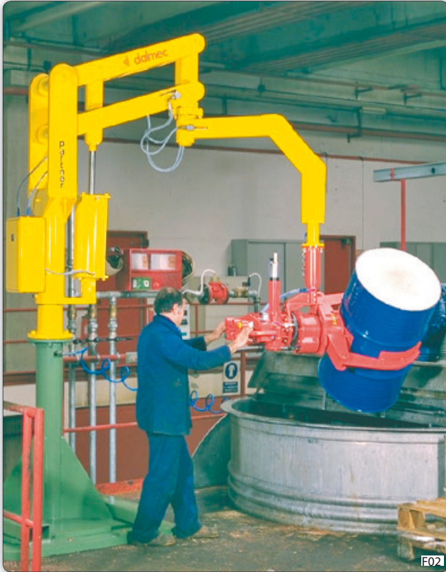
PMC type Partner manipulator, column mounted, made for picking and emptying of drums.
