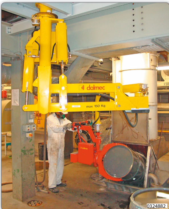
PMF type Partner manipulator, fixed overhead version, designed for the picking and emptying of drums.
