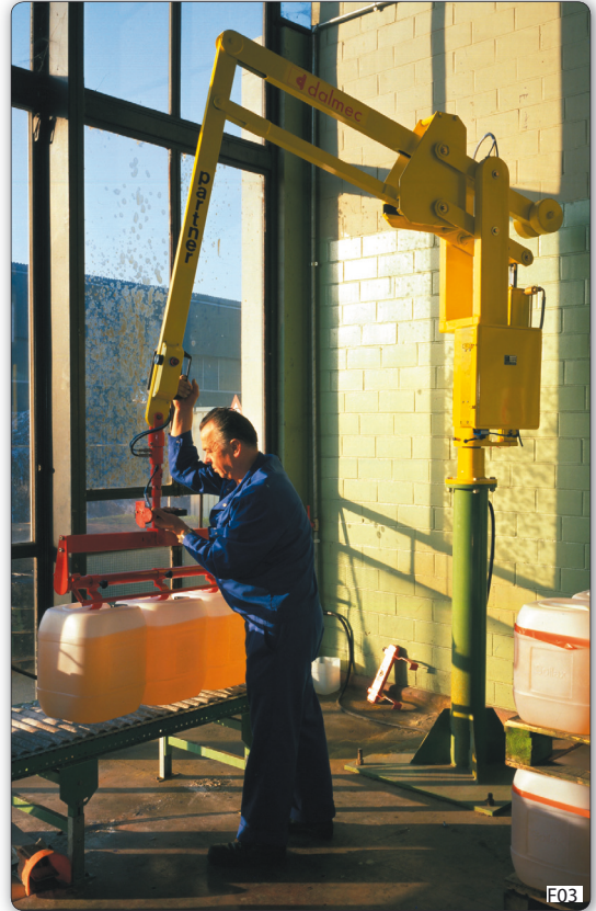
PSC type Partner manipulator, column mounted unit, for handling one or more canisters at once.
