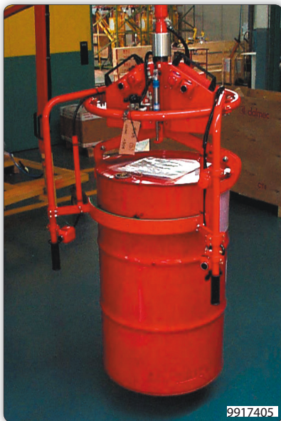
Manipulator with gripper system for picking drums on the rim with dual and low level controls.
