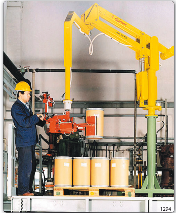
PMC type Partner manipulator, column mounted version, designed for picking and emptying carboard drums.
