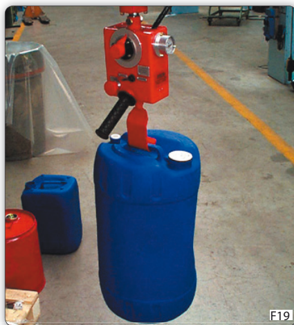
PVC type Posivel manipulator, column design, equipped with specially shaped hook designed for palletizing pails.
