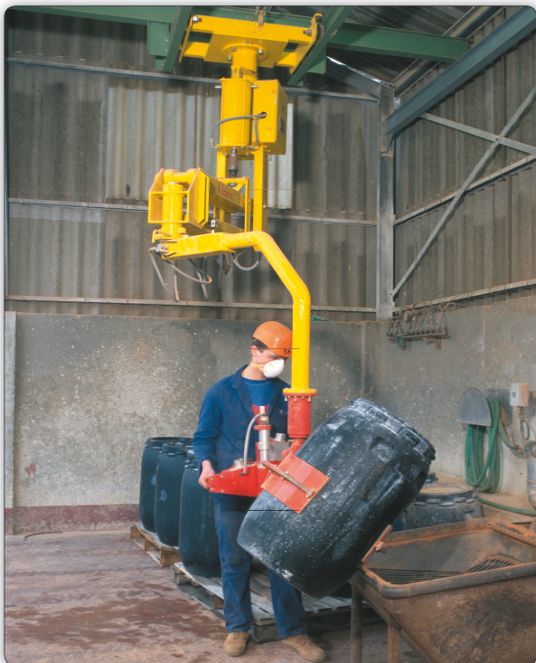
PMS type Partner manipulator, overhead trolley mounted version to cover several work stations, for handling and tipping drums.
