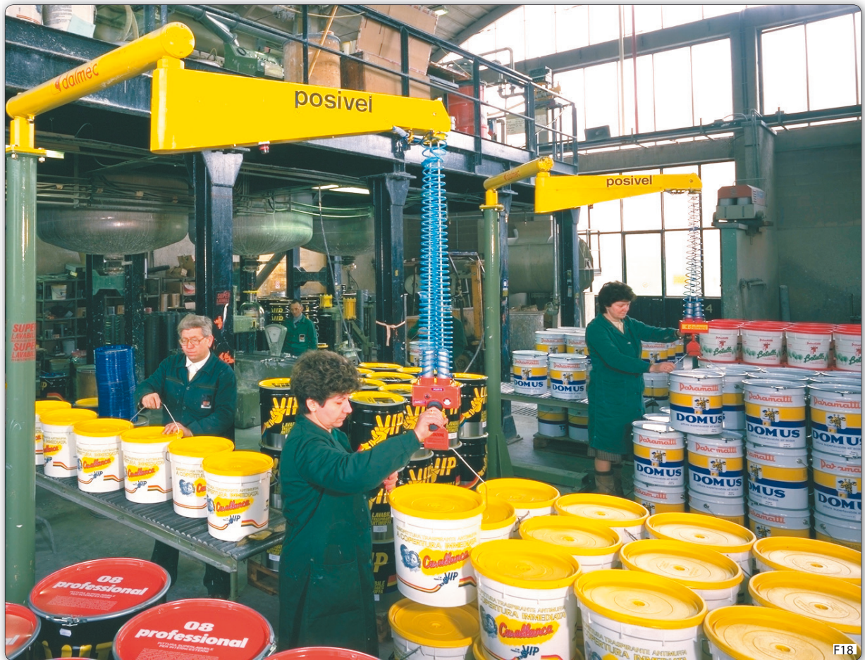
PVC type Posivel manipulator, column design, equipped with specially shaped hook designed for palletizing pails.
