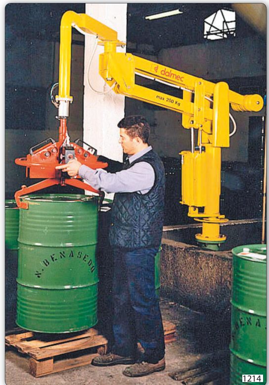
PMC type Partner manipulator, column mounted, equipped with tooling for gripping on the drum's rim.
