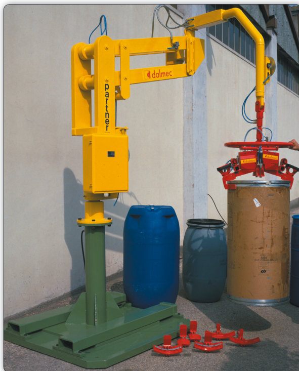
PMC type Partner manipulator, column design, equipped for picking and moving drums of varying shape and weight. Interchangeable grippers are available for handling different sizes of drums.
