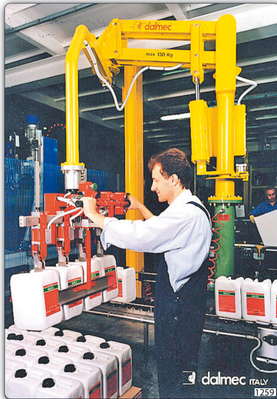
PMC type Partner manipulator, column mounted version, equipped with a pneumatic gripper tooling head to handle four canisters at the same time.
