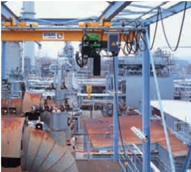
A single girder suspension crane with 1,600 kg S.W.L. is used for transporting components for maintenance work in the outdoor area of a chemical plant.
