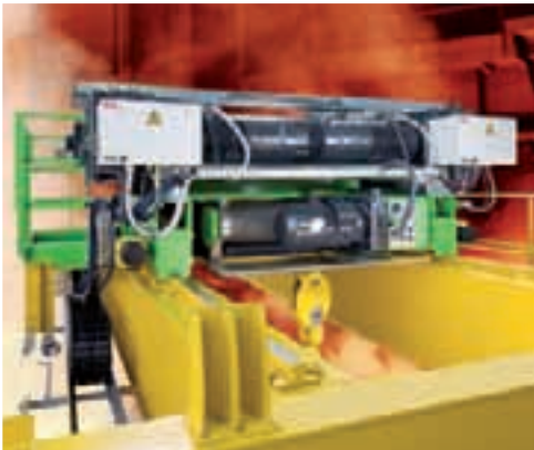
TDC twin drive concept _ doubly safe, for transporting molten metals and similar potentially hazardous goods.
